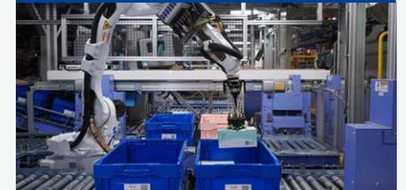
These arm-type robots use 3D-image recognition to automatically generate a movement plan to identify and pick out 2,000 varieties of products.
