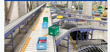
Sorters are controlled by systems to divide products by their outgoing direction and delivery carrier.
